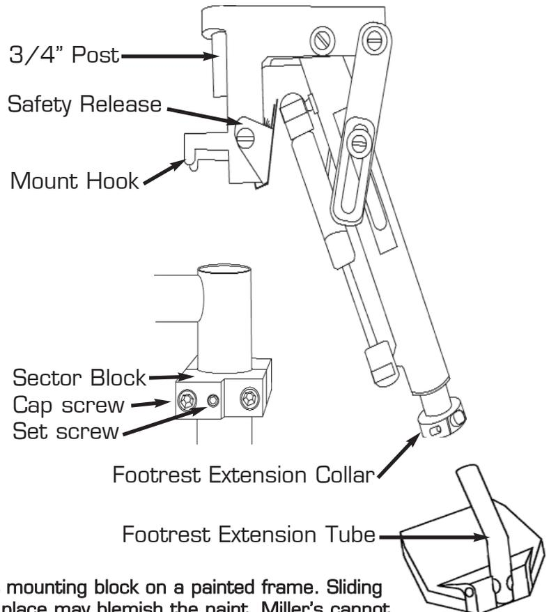
**Caution:** Care should be taken when installing the legrest mounting block on a painted frame. Sliding this device into place or tightening the bolts to secure in place may blemish the paint. Miller's cannot assume responsibility for damage to the paint caused by installing or using this device.
